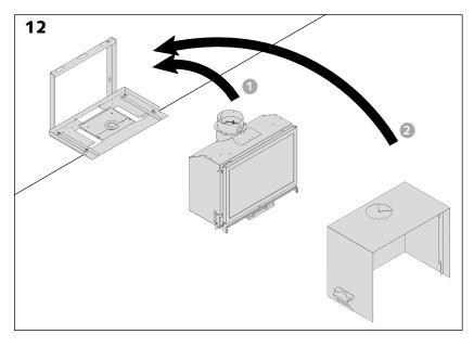
When installing the stove [image 12] refer to the Stûv 16 installation instructions, Chapter "Positioning of the stove".
