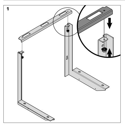
When fitting the pre-installation plate [diagrams 2 & 3], engage the screws but do not tighten them. Final fixing does not take place until the stove has been positioned
