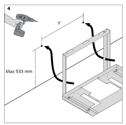
Take care to fix the bracket through the 2 keyholes at the bottom The maximum height measurement is 533 mm.
